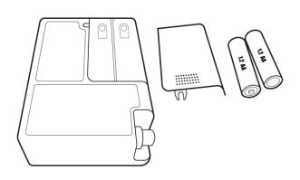
In order to change batteries, take the recorder out of the holder pouch and remove the battery compartment cover on the back-side. Place two properly charged, high capacity AA rechargeable or two new, long-life AA alkaline batteries into the compartment then close it.
